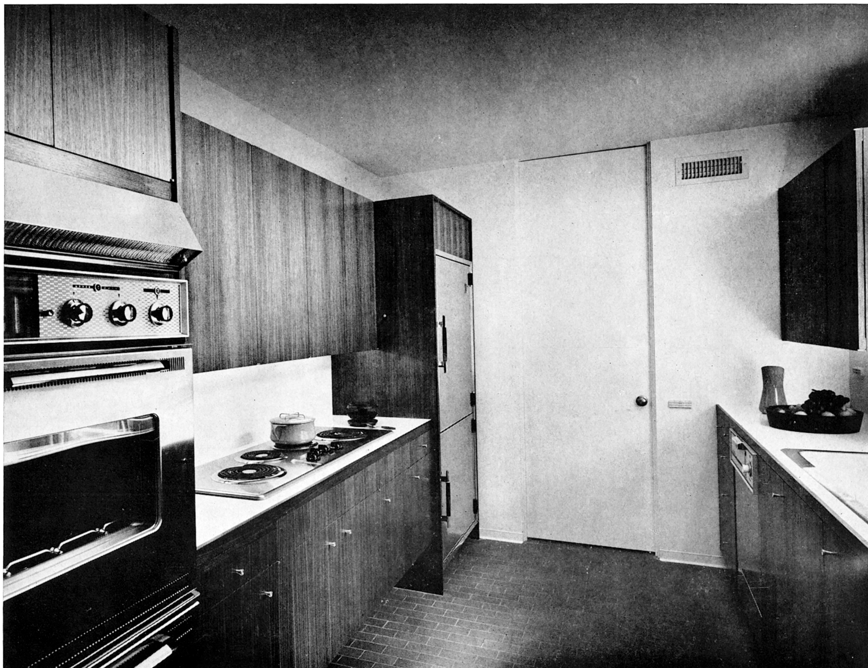
The kitchen toward the south. Thermador ovens and vent to the left, Thermador cook top next to this with a Trade-Wind exhaust fan concealed in the cabinets above. To the right of this, the Revco refrigerator is housed in the cabinet. To the extreme right the sink and Thermador dishwasher may be seen. The Swepe System of light switches is located in line with the door knobs.
