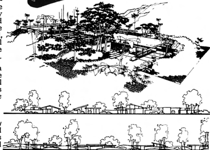
CASE STUDY #24—project in work. 260 houses in a 140-acre tract. Houses to be below grade: individually 'slipped' into excavation. Soil excavated mounded in landscape forms. By A. QUINCY JONES AND FREDERICK E. EMMONS.
